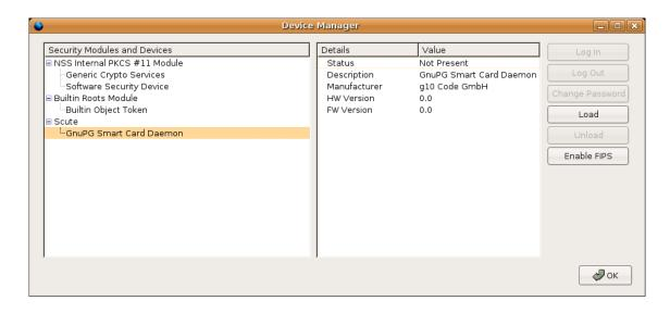
When you insert the OpenPGP card for which you generated and imported a certificate earlier (see Section 2.3 [Certificate Preparation], page 4), the device manager should detect this security token and display some information about it in the Details list when you select it from the module list.
