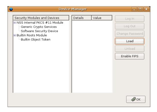
In the pop-up dialog that follows, you can give a module name (e.g. "Scute") and a module filename. The latter should correspond to the full file name of the installed Scute module file scute.so. The default installation path is /usr/local/lib, which would mean that you have to provide the file name /usr/local/lib/scute.so. If you or your system administrator installed Scute in a different location, you have to adjust the file name correspondingly.
